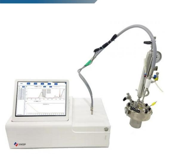
JINSP® IT2000CE online FT-IR analyzer is used for in situ monitoring of chemical reaction. IT2000CE can measure the content of reactants residues, products, intermediates and impurities in the reaction system continuously and quickly, thus predicting reaction rate, reaction termination, conversion rate and reaction incidents in real time.
