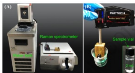
Fig. 1. Photograph of the in-situ Raman monitoring system.
