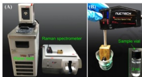
Fig. 1. Photograph of the in-situ Raman monitoring system.
