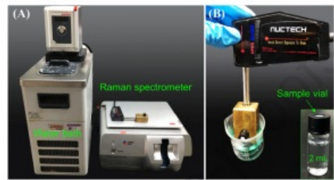
Fig. 1. Photograph of the in-situ Raman monitoring system.
