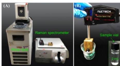
Fig. 1. Photograph of the in-situ Raman monitoring system.
