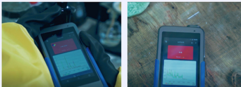
The RS1500 detects liquid and small particle (panel interface can be switched to multiple languages)
