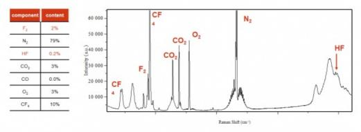
**Application: 2.** Quantitative analysis of different Elements in Petrochemical Natural Gas Effective identification and quantification of various components in natural gas mixtures within 2 seconds, such as alkanes, alkenes, alkynes, etc.
