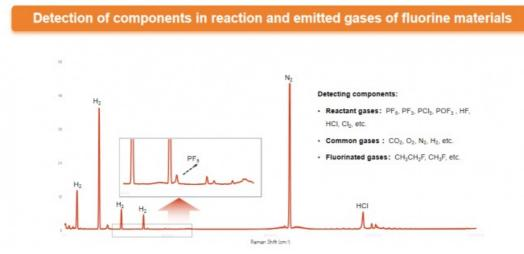
Application: 4. Detection of impurity gases and electronic special gases.
