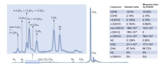
Effective identification and quantification of various components in natural gas mixtures within 2 seconds
