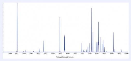
Test results and applications in the range of 200~1000nm-Mercury-Argon Lamp Spectrum
