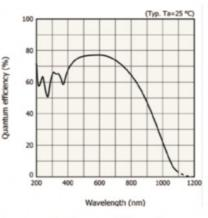
**CCD Quantum Efficiency Curve**
