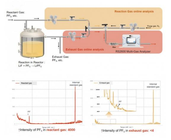
This Online Analysis Solution Enables:1. Real-time, in-situ, continuous monitoring of multiple components in reactant gases and exhaust gases.2. Determination of reaction endpoint!
