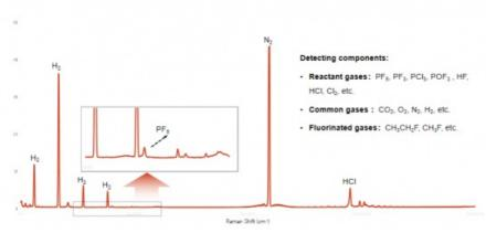
Application: 4. Detection of impurity gases and electronic special gases.
