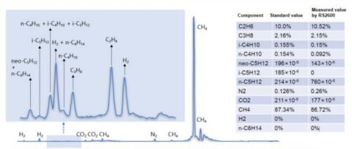
Effective identification and quantification of various components in natural gas mixtures within 2 seconds
